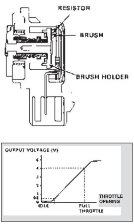
The throttle position sensor on a speed-density system works just like the corresponding sensor on most other fuel injection systems, with a varying return voltage depending on the position of the throttle pedal. This sensor also provides information about the speed of throttle plate movement to the computer.
