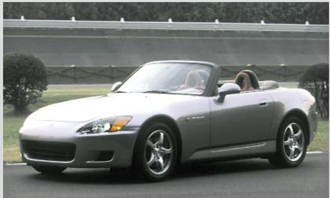
Honda S2000 convertible has a 2.0 liter four-cylinder that produces 240 horsepower, the highest output per liter of any naturally-aspirated engine. The S2000 six-speed manual gearbox is taken from the Acura NSX.
