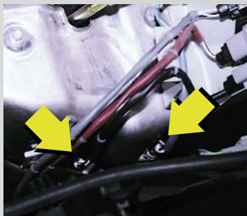
Figure 3: The Sentra 1.8-four has four oxygen sensors, two at top as indicated.
