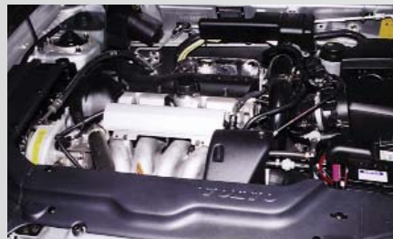
Figure 18: Volvo 40 series has a 1.9 liter turbo, and it too has a timing belt with the upper cover held by spring clips for inspection access to the belt.
