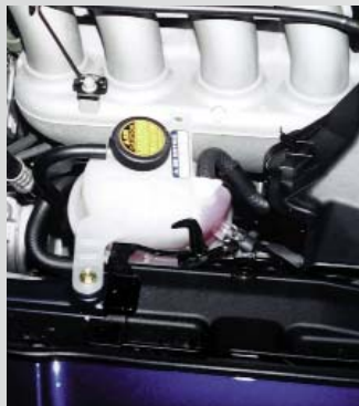
Figure 9: With the Celica beauty cover off, you can see the pressurized coolant reservoir. In this aerodynamic front-end model, the reservoir is not at the high point of the cooling system, so it has to be unbolted and raised (also freeing some hoses after loosening the air cleaner cover). The reservoir can rest on the hood latch.
