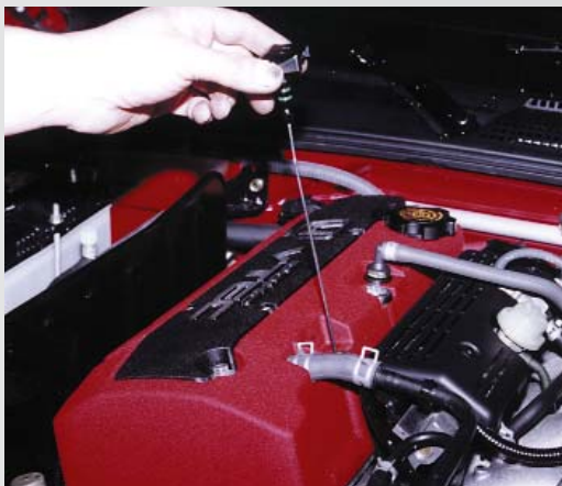
Figure 21: The oil fill cap also holds the dipstick. As you can see, the dipstick goes all the way through the engine down to the oil pan.
