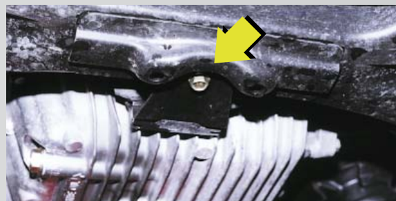
Figure 22: Don't jack up car by the control arms. In front, use this reinforcement (or the reinforced areas on the longitudinal rails, provided for the scissors jack).
