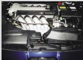
Figure 8: Celica powertrain compartment has the usual gray 'beauty' covers, and the coolant reservoir is under the one on the right side.
