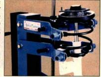
ing compression, a double-lead center screw keeps the strut and spring aligned — no matter what shape the spring has. The double-lead screw also compresses the spring faster than any comparable model. The tool mounts easily to a workbench or the wall because there is no mounting hardware. There's also a stand with a welded steel frame and two wheels to move the entire unit around the shop as needed.
