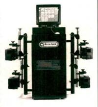
software and ALLDATA Undercar software. Four CCD headsallow quick and precise measurements of caster, camber and toe angles for all four wheels. A 17-inch monitor displays operating instructions, readings and three-dimensional adjustments. The system fits in a compact cabinet mounted on casters.
