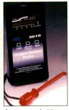
firm operation of the feedback system. A 20-segment bar graph indicates rich or lean, and the tool measures the activity level of the sensor to discover 'lazy' or inert sensors. An LCD display shows crosscounts. The tool works on a 9-volt battery, eliminating the need for power leads. It shuts itself off automatically.
