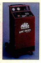
high and low sides for increased speed. Then an electronic scale weighs the amount of refrigerant recovered and accurately recharges the vehicle's system by weight. A special filter-drier removes oil and contaminants from the refrigerants, and an automatic air purge removes air contamination during the vacuum/recycling process.
