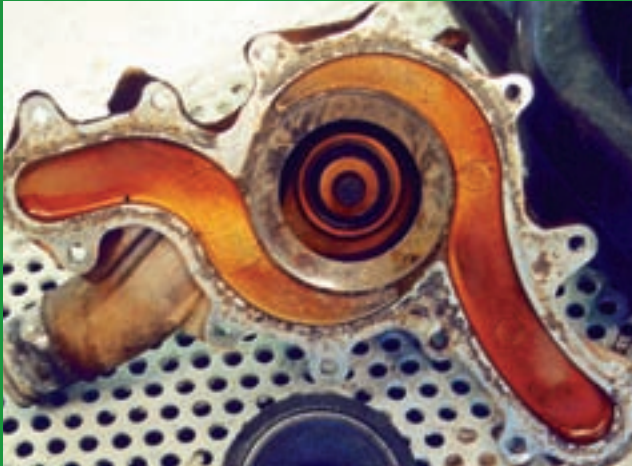
Damaged Water Pump
