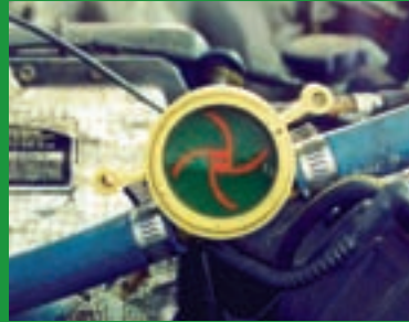
Measuring Coolant Flow
