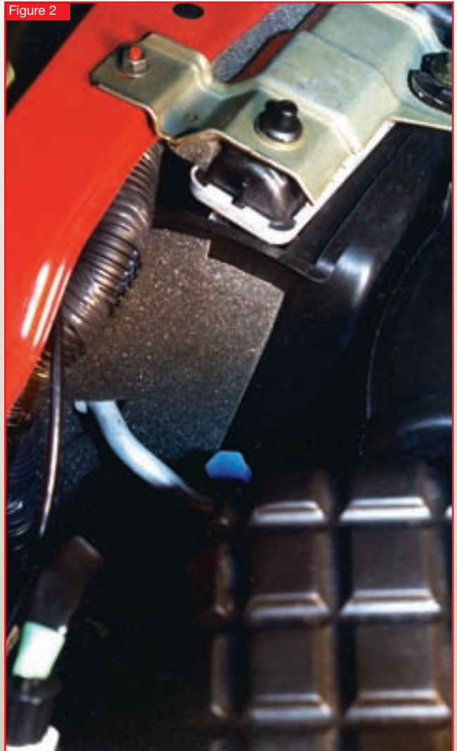
This Frontier engine compartment view shows a foam seal at the headlamp openings, another one is installed for A/C and cooling.
