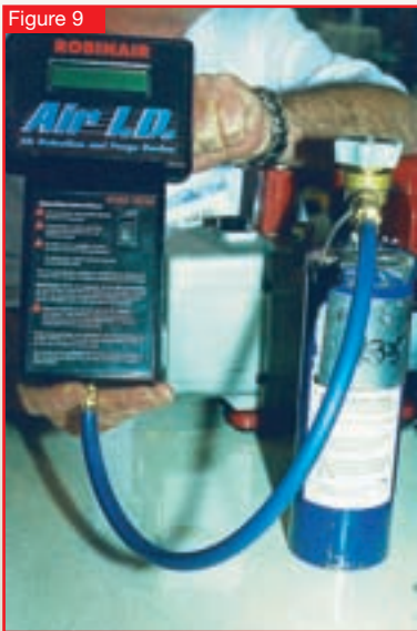
Robinair's Air ID attaches to the recycled refrigerant jug and gradually purges it, checking for air automatically every hour. The Neutronics Air-Radiator, a more expensive machine, is also designed for limited air-purging of vehicle systems.
