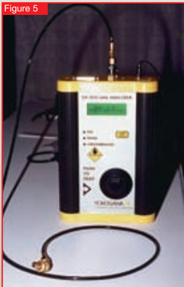
Yokogawa’s new identifier also is in the 98 percent accuracy range, and can operate on 12-volt DC, 110-volt AC, and an optional battery pack.
