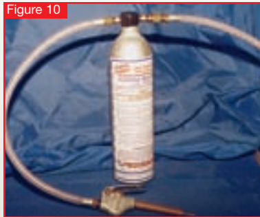
A simple flush gun, plus collection tank and hoses are all you need to flush systems with R-141b. You may already have this flush gun in your shop.
