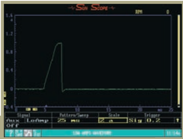
Figure 5 Low Current Amp Probe Waveform Of A Saturated Switch-type Injector
