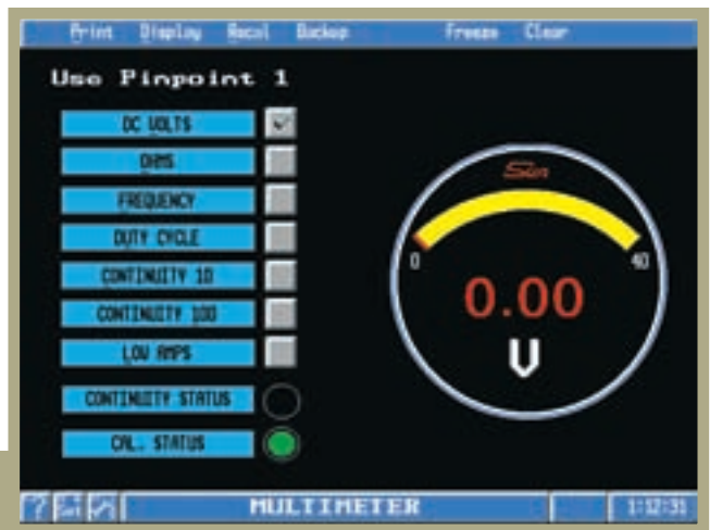
Figure 2 DC Volts Display
