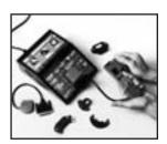
replaced ignition modules. It's the only tester on the market that can test the inductive modules used by most import car manufacturers, says Innova, and it's easily upgraded to test new modules as they are introduced.
