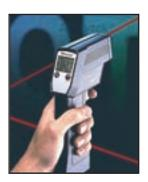
backlit display is easy to read and laser sighting provides pinpoint accuracy, especially in dim light conditions. A protective hard case is included with every unit. The Raynger ST may be used in a variety of automotive applications. Automotive technicians can measure inlet and outlet temperatures of catalytic converters, mea-
