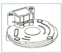
An erratic spark and fuel injection control condition on mid-eighties Nissan vehicles that goes away as the vehicle warms up may be caused by the presence of oil on the optical crank an-
