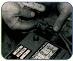
We disconnect the battery first thing. If we do have a shorted harness, we'd rather not find the problem area by backtracking to the source of smoke! We also take the time to clean the battery, battery posts and terminal ends for later installation. Every car should get this treatment at least once in its life.
