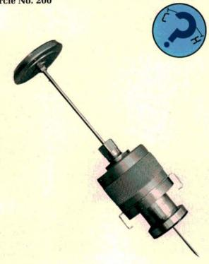
Each probe fits through a diaphragm in the adapter. As you remove each probe to install another, the diaphragm automatically seals itself, preventing any loss of coolant. Changing probes is as easy as removing one probe and inserting another without the need to remove the adapter from the radiator.
