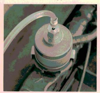
You want to run another pressure test now that the cooling system is hot? Remove the temperature probe and reinstall the pressure probe. The tester allows you to bounce back and forth between tests without opening the system. After completing tests on a hot system, vent the system pressure by inserting this vent probe, and catching the hot overflow in a suitable container.
