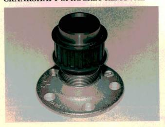
My tech tip relates to the "Tension Headache" article in the July 1991 issue of *Import Service*. I have found that two pieces of pipe can be used to safely remove the Toyota 5M-GE engine's crankshaft timing sprocket.
