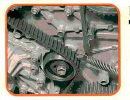
Make sure the crankshaft is still at TDC. Relieve the timing belt tension by loosening the belt tensioner pulley set bolt. Prop a screwdriver against the long bolt in the inner cover, then push the pulley toward the alternator. Retighten the pulley set bolt. Slip the belt off the cam sprockets.
