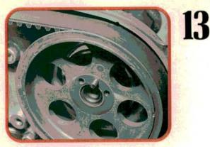
Recheck the camshaft match holes, cam sprocket timing marks, and crank pulley TDC mark for proper alignment. Look through the three holes at the front of the cam sprockets. Select one hole in each sprocket that aligns with a matching hole in the camshaft, then install the match pin.
