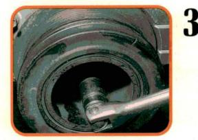
Remove the idler pulley and A/C compressor bracket. The bracket wraps around the front of the lower timing cover. Remove the crankshaft pulley bolt, then the crankshaft pulley. Our pulley wiggled off by hand, you may need to use a puller. Remove the lower timing cover bolts and cover.
