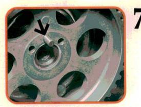
Setting the cam timing is a little different on the 5M-GE. Each camshaft sprocket has three alignment holes, and three mating holes in each camshaft. The hole spacing is offset, so only one camshaft and one sprocket hole will line up at a time. A match pin fits between them to hold the adjustment.
