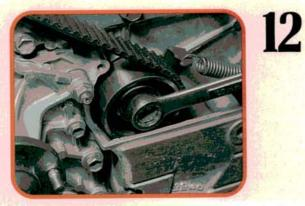
Loosen the tensioner pulley set bolt and allow the tensioner spring to remove the timing belt slack. Belt tension between the exhaust camshaft sprocket and the tensioner pulley should be equal to the tension between the intake camshaft sprocket and oil pump drive sprocket.
