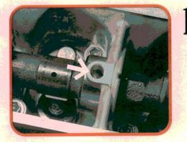
Turn the crankshaft until the intake camshaft and cam housing match holes are aligned. Check the position of the crank pulley pointer. Now align the exhaust cam match holes. The crank pulley pointer must be within 5 degrees of TDC when each pair of cam match holes is aligned.
