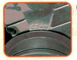
Slip the new timing belt over the crankshaft sprocket. Reinstall the lower timing belt cover and drive belt pulley. Apply thread locker, then torque the crank pulley bolt to 197-235 Nm (146-174 ft-lb). Reinstall the A/C compressor bracket. Align the crankshaft pulley notch with the zero degree timing mark.
