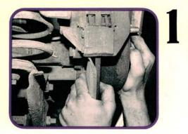
To check the lower trailing arm bushings, raise the car on a frame contact hoist so the rear axle hangs free. Now push up on each end of the rear axle from below. You'll be able to feel the looseness in the suspension if the lower trailing arm bushings are worn.
