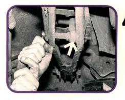
Normally the next step would be to remove the lower shock mounting bolt from the trailing arm. The underside of this Volvo had seen over 80,000 miles of northeastern Ohio weather, so we didn't expect it to be easy. The lower shock bolts on both trailing arms were rusted solid to the lower shock bushings.
