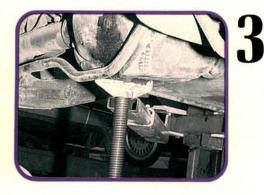
Support the rear axle housing with a jack stand. The trailing arm can't be lowered far enough to get at the trailing arm bushing unless the rear shock is disconnected first. The rear shocks limit the rear suspension's downward travel, so the stand is needed to keep the axle from dropping too far.
