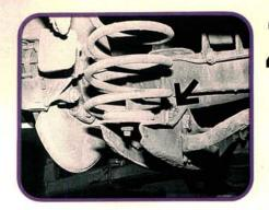
The lower trailing arm bushings are pressed into mounting ears on the underside of the axle housing (arrow). The trailing arm, shock absorber, sway bar, and coil spring must be disconnected and lowered out of the way to replace the bushings. We found it easier to replace the bushings one side at a time.
