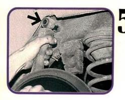
There are a couple of options in this situation. If the rear shocks need replacement anyway, cutting the rusted lower shock bushings with a torch only takes a few extra minutes. The shocks were still good in this car, so we disconnected the upper shock mounting nut instead.
