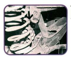
The outer bushing mounting ear has a smaller inside diameter than the inner ear, so the bushing must be removed by driving it toward the center of the car. Working at the center of the bushing, use the air chisel to carefully push the caved-in bushing to the right.
