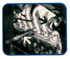
This photo will give you a better view of some of the things you can only find by feel while the head is still in place. The spring-tensioned oil by-pass breather hose is attached to the head (white arrow). The heater hose we removed at the firewall is still attached to the manifold (black arrow).
