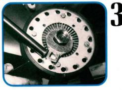
The cooling fan screws onto the threaded water pump shaft with a LEFT-HAND thread. Take a 32 mm or 1½ inch crows foot, and strike the head of the wrench with long bar to break the fan free. Unscrew and remove the fan. Radiator removal is not necessary, but you'll need to drain the coolant.
