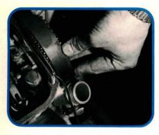
Double check your timing marks. Install the new belt. If the belt teeth don't fall right into the notches on the camshaft sprocket, bump the cam to the nearest tooth that fits. Make sure the belt teeth are sitting square in the crank sprocket. Keep the side of the belt away from the tensioner pulled tight.
