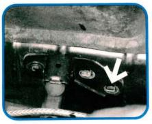
Start by removing the hood. Disconnect the windshield washer fluid hose and plug it. Spray paint the bolts in the hood hinges before you remove them. That way, you can use the paint marks as bolt locators when you reinstall the hood, and be right on the money the first time.
