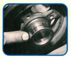
Remove the front pulley. Clean it and inspect the surface where the front crank seal rides. Leaking oil from a heat-hardened seal will mix with dirt to form an abrasive paste that will eventually ruin the pulley sealing surface. This pulley showed a small amount of wear, but was reusable.
