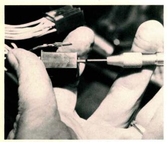
Sliding Resistance Test—Subaru
