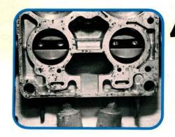
Soaking the carburetor may loosen dirt and deposits in the internal passages. Take a little extra time to make sure that they are all clean and clear. The two idle shutoff solenoids also control the flow of fuel to the primary main jets. Test both solenoids electrically for proper operation.
