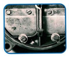
The two rear air horn screws extend through to the throttle base. Each screw should have a flat washer under its head. These should prevent damage to the air horn. Point the tabs on the washers toward the notches in the air horn. Install the six remaining air horn screws, then tighten the two base screws.
