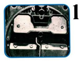
Dismantle the carburetor completely. Remove any diaphragms or other rubber parts that might be damaged by carburetor cleaning solvent. Soak the carburetor only long enough to remove the dirt. Oversoaking may cause damage to the rubber o-rings that seal the emulsion tubes to the carburetor bowl housing.
