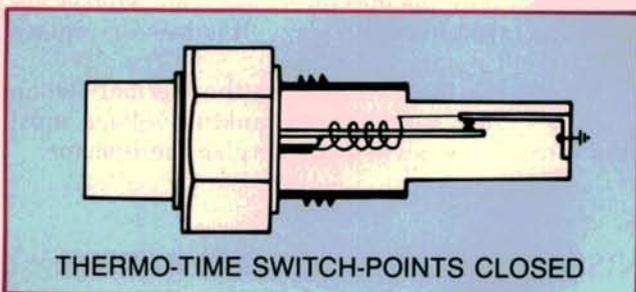
The same current used to energize the starter solenoid in the crank position also feeds the time switch and cold start injector. It travels to the cold start injector to energize it. It also travels through a heating coil wrapped around another bi-metallic spring, similar to the one found in the control pressure regulator. A set of contact points on the bi-metallic arm connect it to ground. Ground is also supplied to the cold start injector as long as the points in the time switch stay closed.
