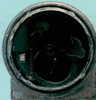
As you can see, the heart of this system is fuel pressure. There's precious little electricity involved in basic K-Jet, and the need for a good vacuum source to lift the sensor plate is not radically different from most other fuel systems.
