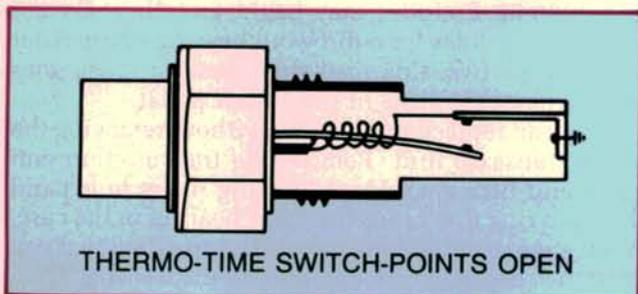
As a result, we have crank voltage and ground supplied to the heating coil and the cold start injector. The heating coil warms the bi-metallic spring causing it to deflect slightly. This movement opens the points, eliminating the ground circuit to both the switch heater and injector.
